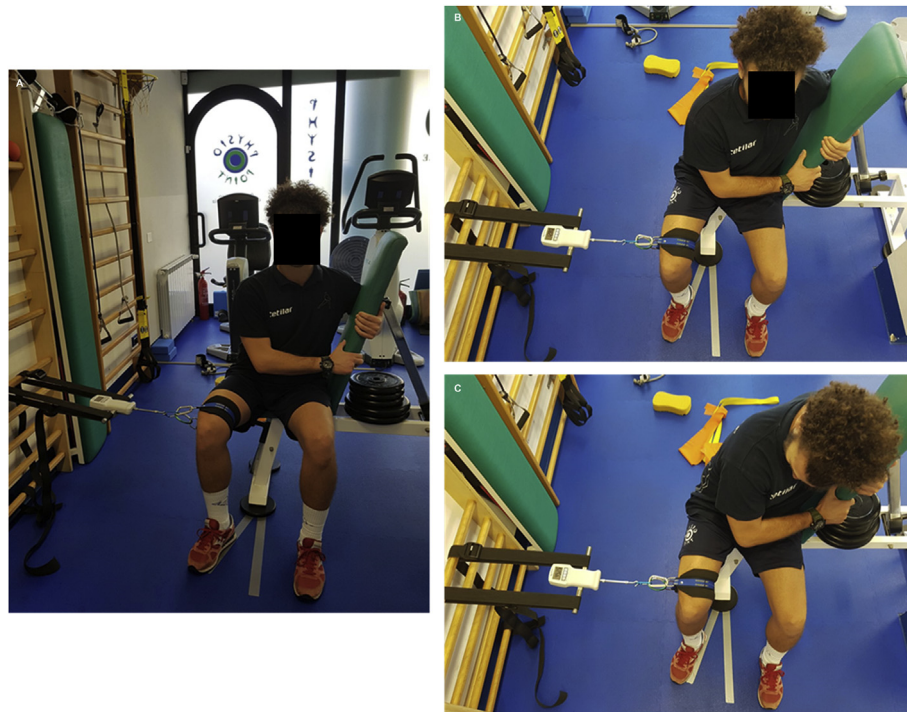
Figure 5. Strength test. The photos represent how the strength test was performed. Panel A shows the position of the professional roller hockey player at rest holding the backpad. Panel B shows the position of the leg opened at 20°. Panel C shows the professional roller hockey player during the test.
